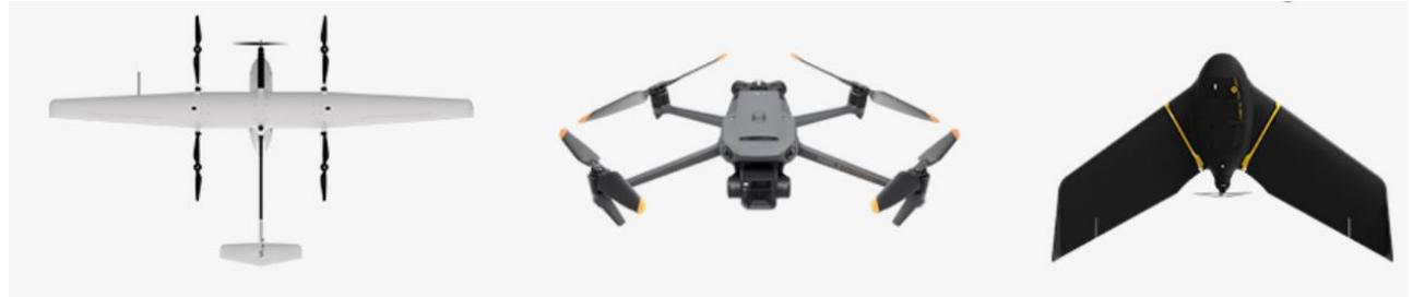
**Vertical Take-off and Landing Drone vs Multirotor Drone vs Fixed-wing Drone**
